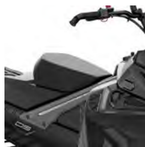
DEEP SNOW PRO SEAT 860202264 Provides greater freedom of movement. Low, narrow and light seat. Integrated grip areas. RADIEN RADIEN-X 400 MM
