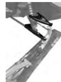
A-ARM WIDENING KIT 860202194 Provides more stability when turning on steep slopes. Adds 200 mm of width to the front suspension. 59 & 69 RANGER ALPINE
